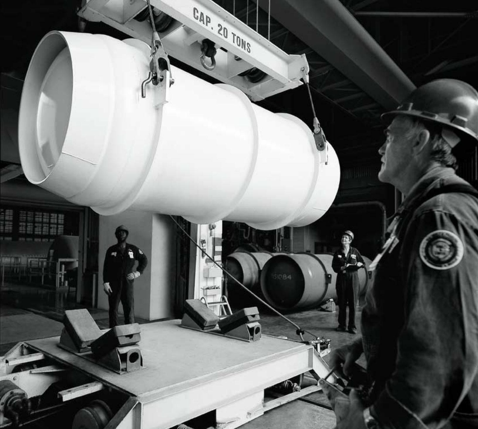
Jerry Neale (foreground), Curly Ware (left) and Donna Shelton prepare to weigh a cylinder of UF 6 upon its arrival at the plant.
