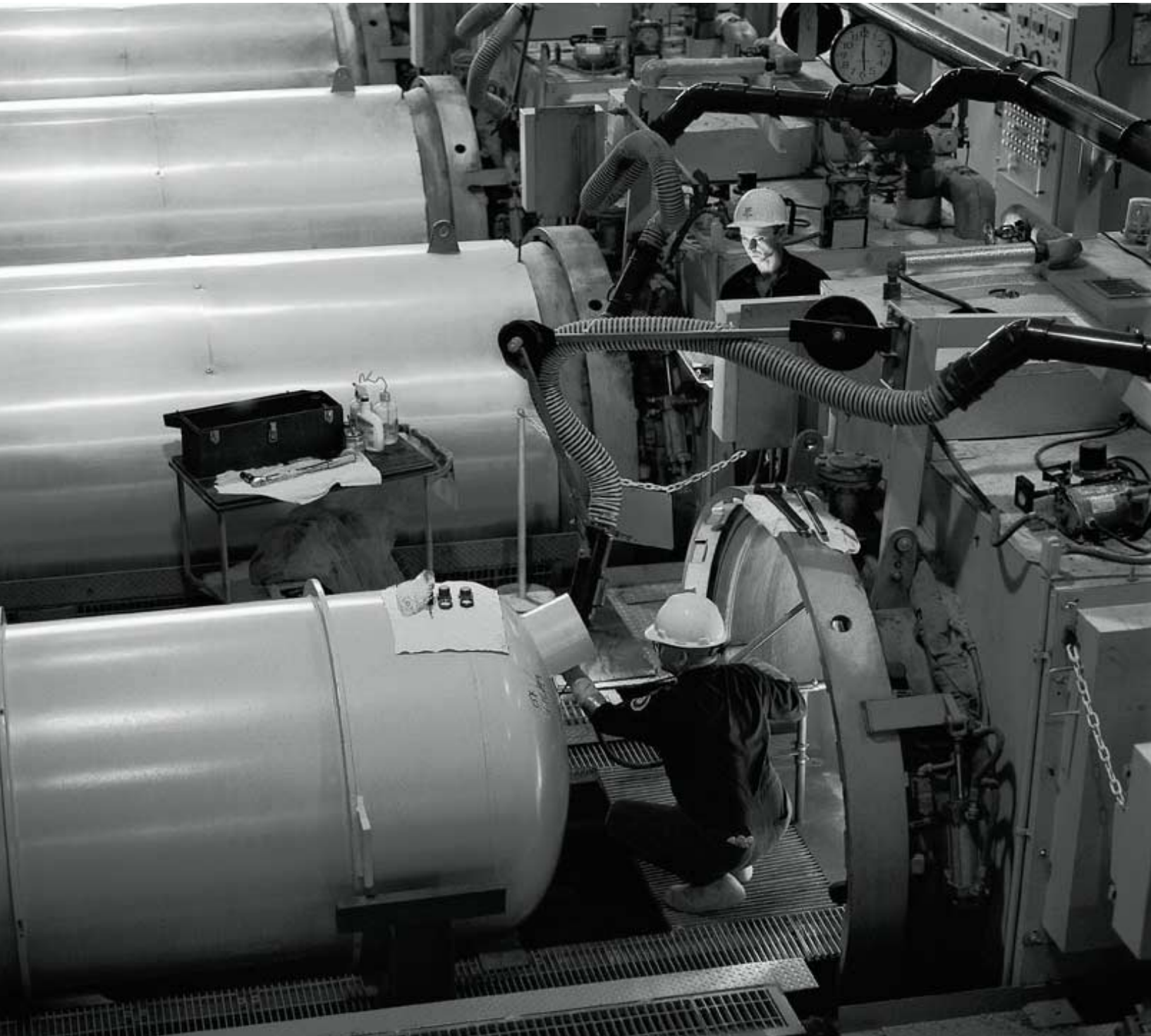
Troy Karnes (top) and Freddie Thompson prepare a cylinder containing UF 6 , which will be heated and introduced into the gaseous diffusion process.
