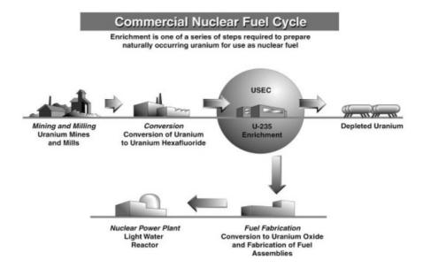
The standard measure of uranium enrichment is a separative work unit ("SWU"). A SWU represents the effort that is required to transform a given amount of natural uranium into two streams of uranium, one enriched in the U<sup>235</sup> isotope and the other depleted in the U<sup>235</sup> isotope. SWUs are measured using a standard formula derived from the physics of uranium enrichment. The amount of enrichment contained in LEU under this formula is commonly referred to as its SWU component.
