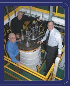
Development of the American Centrifuge uranium enrichment technology passed an important milestone in April 2005 when USEC began manufacturing centrifuge components. The American Centrifuge team built full-size prototype centrifuge machines that are being evaluated in highly specialized test equipment in Oak Ridge, Tennessee.
