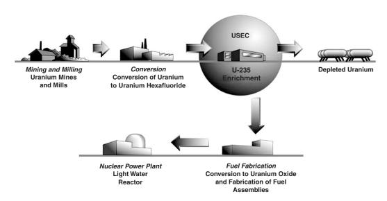
We produce or acquire LEU from two principal sources. We produce LEU at the gaseous diffusion plant in Paducah, Kentucky, and we acquire LEU by purchasing the SWU component of LEU from Russia under the Megatons to Megawatts program.
